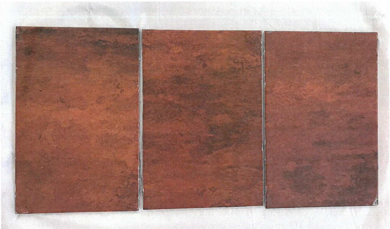
Photo 3. HPDE coating after AASS Test.
