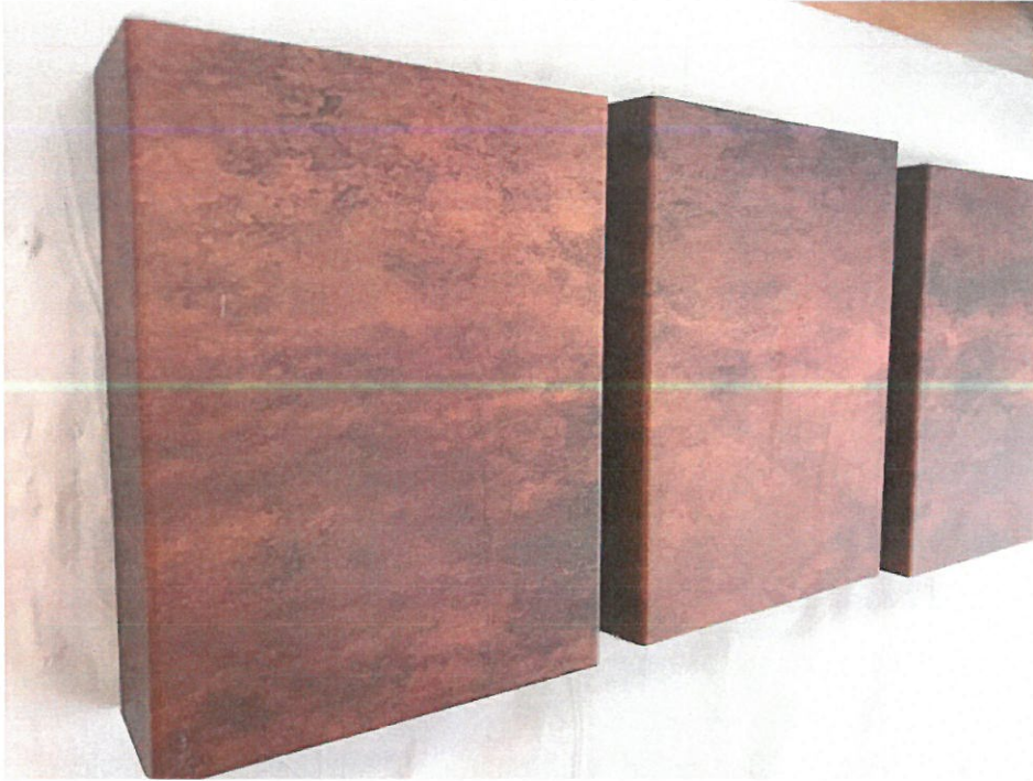
Photo 2. HPDE coating after AASS Test.
